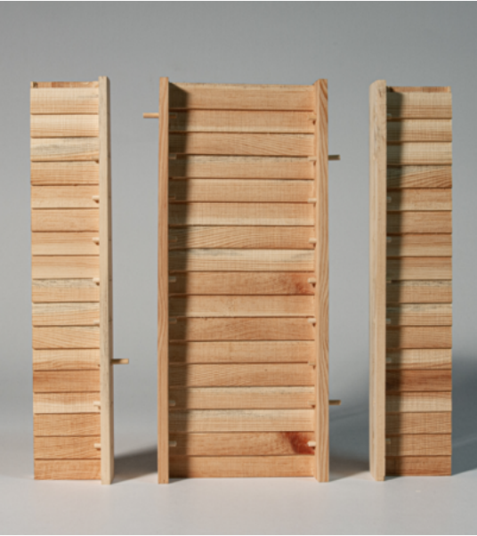
1:20 CLT panel disassembled
