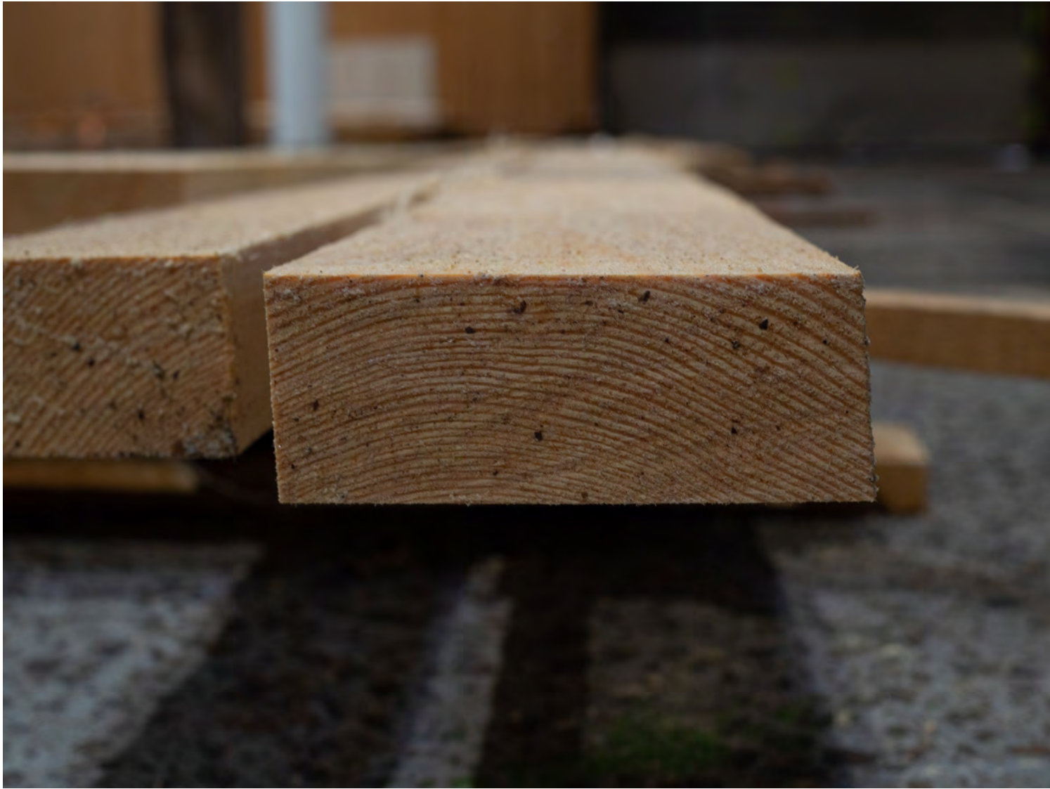
The timber is cut in different dimensions to accommodate different needs as paneling, structural purposes, stiffening and cladding. The boards are mounted together without adhesives or metal, but with wooden nails.
