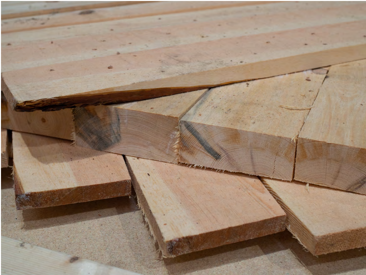
The timber is cut in different dimensions to accommodate different needs as paneling, structural purposes, stiffening and cladding. The boards are mounted together without adhesives or metal, but with wooden nails.
