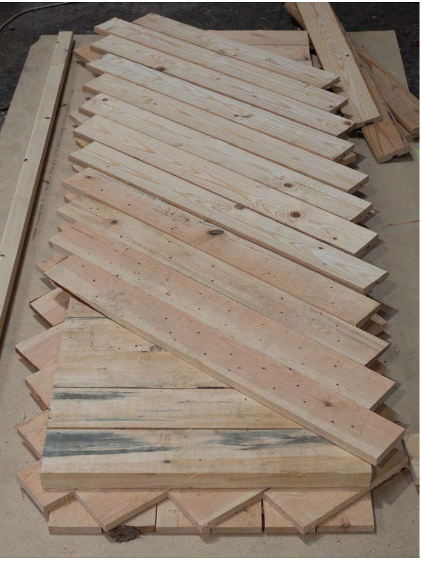
Two of the total of five layers are diagonal to provide stiffness and the core boards are slightly thicker to allow for better load bearing and thermal properties.
