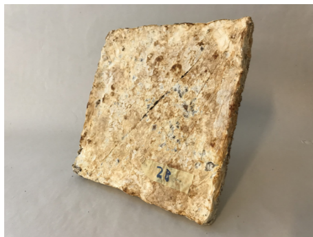
Accoustical plates grown with different substrates.
