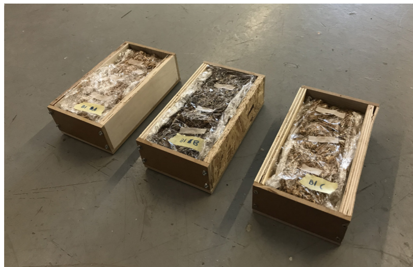
Mycelium bicks in the making, using spent mushroom substrate (2023)
