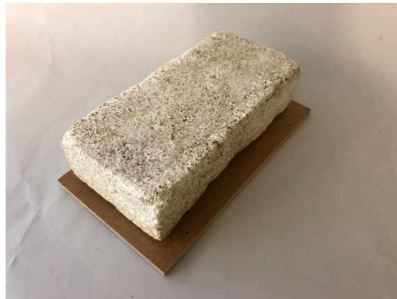
Mycelium brick using SMS (2023)
