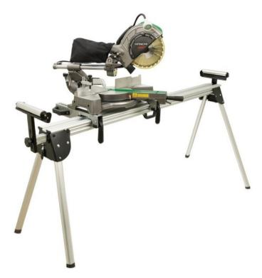
This saw is used in the workshop and on projects in the field. It is a portable non-handheld machine. A mitre saw is a highly versatile and accurate tool used to cut and adjust wooden materials. The saw can be set to a range of different angles by tilting the blade and/or rotating the turntable. The largest models are capable of cutting very wide and high workpieces. The depth of the kerf can also be adjusted to allow you to cut shoulders or rebates in the workpiece.
